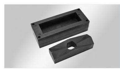
Rectangular and square punches and dies make it easy to punch holes into stainless steel (V2A versions), mild steel, aluminium or plastics with a max. sheet thickness of 2 mm. Available for cut-outs sizes of 10-, 16-, and 24- multi-pin heavy industrial connectors and also for numerous special cut-outs. Therefore, the punches are suitable for most icotek cable entry systems. Centre punches are integrated in the die for exact drilling of mounting holes.
